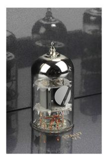
A 12AU7 double triode; six valves/twelve triodes in all are used. Typical life time is 10,000 hours and they are inexpensive.
